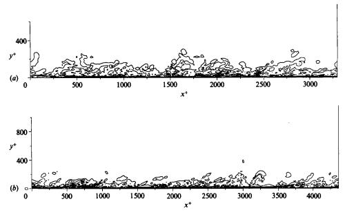
FIGURE 11. Vorticity contours in a streamwise vertical plane. Flow from left to right. (a) Constant-pressure flow,  $R_{\theta} \approx 600$ ; (b) sink flow,  $R_{\theta} = 690$ .
