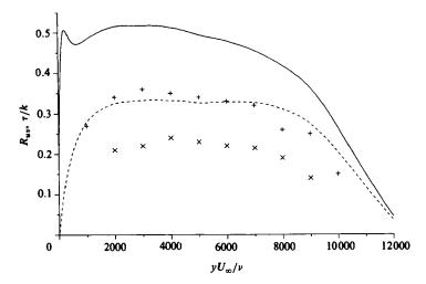
FIGURE 7. Correlation coefficient and structure parameter.  $K=1.5\times 10^{-6}$ . Present results: —. correlation coefficient; ——, structure parameter. Jones & Launder: +, correlation coefficient;  $\times$ , structure parameter.
