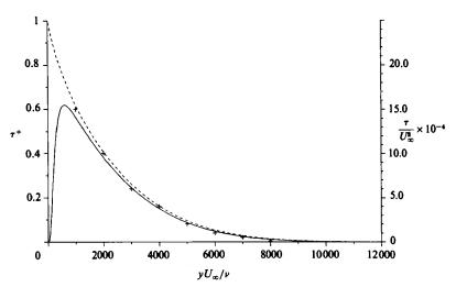
FIGURE 5. Shear stresses,  $K = 1.5 \times 10^{-6}$ . Present results:—, Reynolds stress; ---, total stress. Jones & Launder: +, Reynolds stress.
