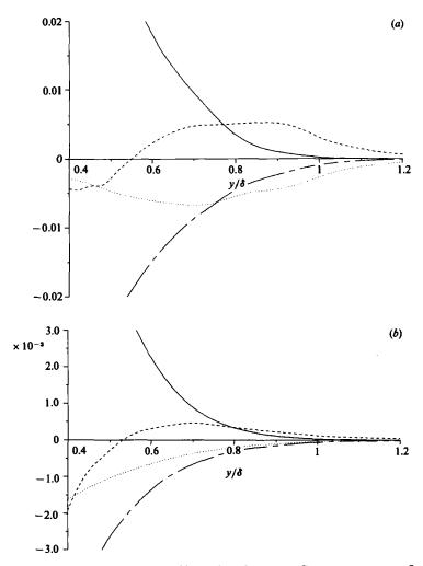
FIGURE 10. Energy balance near edge of boundary layer. (a) Constant-pressure flow,  $R_{\theta} \approx 600$ ; (b) sink flow,  $R_{\theta} = 690$ . —, Production; ——, dissipation; ···, advection; ——, diffusion. Normalized by wall units.
