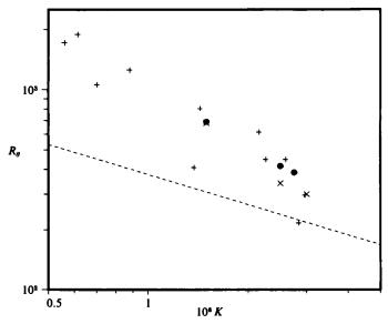
FIGURE 1. Momentum-thickness Reynolds number as a function of the acceleration parameter: ---, laminar flow; ●, present results; ×, Jones & Launder (1972); +, other experiments (see Jones & Launder 1972).
