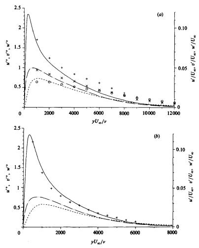
FIGURE 6. R.m.s. of velocity fluctuations. (a)  $K = 1.5 \times 10^{-6}$ , (b)  $K = 2.5 \times 10^{-6}$ . Present results; —, u'; ——, v'; ——, w'. Jones & Launder: +, u';  $\bigcirc$ , v',  $\times$ , w'.
