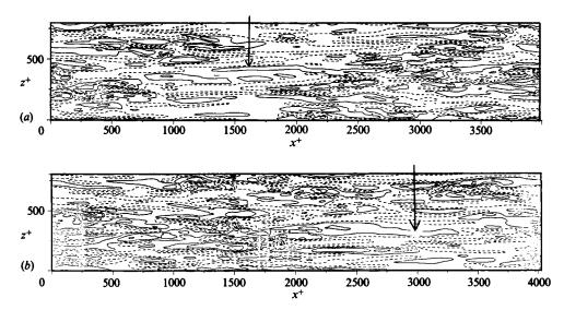
FIGURE 14. Streamwise velocity contours in horizontal plane,  $y + \approx 11$ . Flow from left to right.  $K = 2.5 \times 10^{-6}$ . —, higher than mean; ——, lower than mean. (a) time  $t_0$ ; (b) time  $t_0 + 2060\nu/(U_\infty u_\tau)$ .
