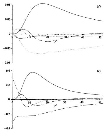
FIGURE 13. Reynolds stress balances near the wall.  $K = 1.5 \times 10^{-6}$ . —, Production; ——, dissipation; ···, pressure diffusion; ···, viscous diffusion; ···, turbulent diffusion. The contribution of the growth terms is insignificant. All terms normalized by wall units. (a)  $u'^2$ ; (b)  $v'^2$ ; (c)  $w'^2$ ; (d) -u'v'; (e)  $(u'^2 + v'^2 + w'^2)$ .
