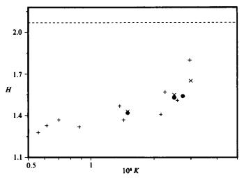
FIGURE 2. Shape factor as a function of the acceleration parameter. ---, laminar flow;
