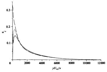
FIGURE 12. R.m.s. of vorticity fluctuations,  $K = 1.5 \times 10^{-6}$ . —,  $\omega_x'$ ; ———,  $\omega_z'$ ; ———,  $\omega_z'$
