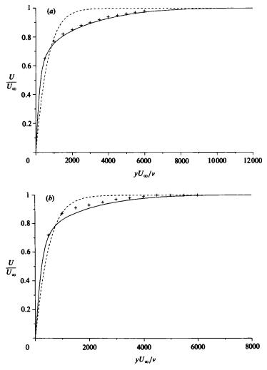
FIGURE 3. Mean velocity profile. (a)  $K = 1.5 \times 10^{-6}$ ; (b)  $K = 2.5 \times 10^{-6}$ . ---, laminar flow; --, present results; +, Jones & Launder.
